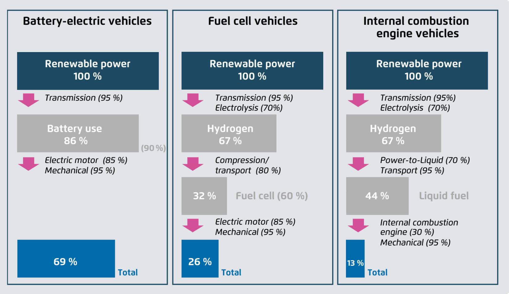
→ To travel the same distance, a **combustion-engine vehicle** would need about **five times** as much renewable electricity as a battery-driven vehicle.
